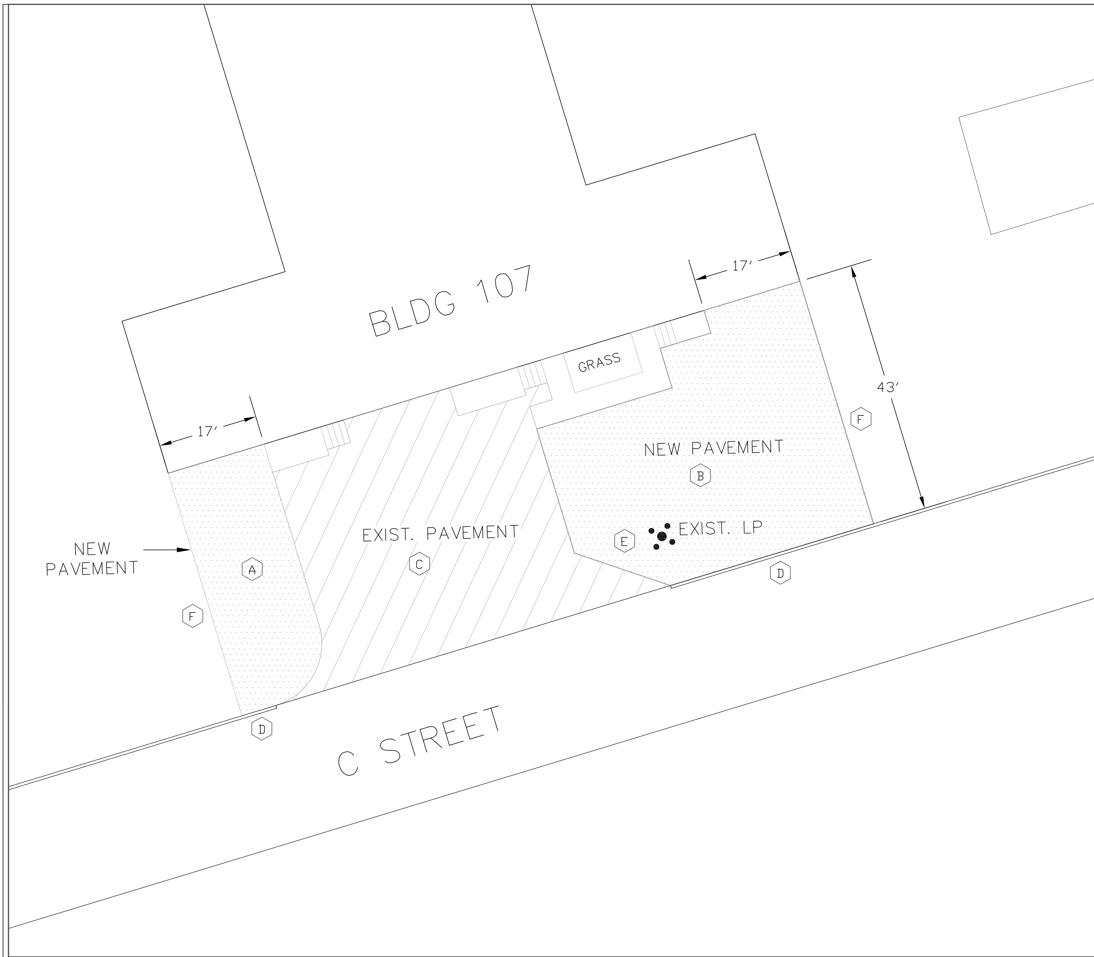
SITE PLAN BLDG 107 PARKING AREA
